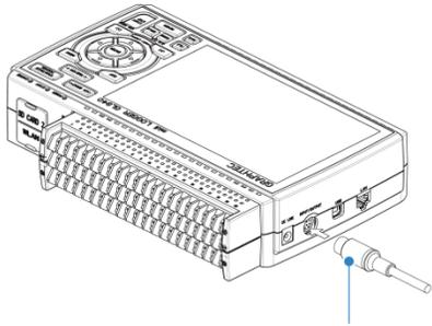
Input/output cable for GL (B-513: Option)
